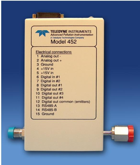
The Model 452 is a microprocessor-based gas sensor for measuring high concentrations of ozone in oxygen or air with accuracy and dependability. The measurement principle is based on the absorption of UV light at 254nm.
