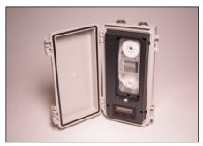
The microAeth® MA350 is a real-time 5-wavelength UV-IR Black Carbon monitor housed in an outdoor-rated case with an 85 sampling location automatic filter tape advance system which allows for 3-12 months of continuous measurements.
