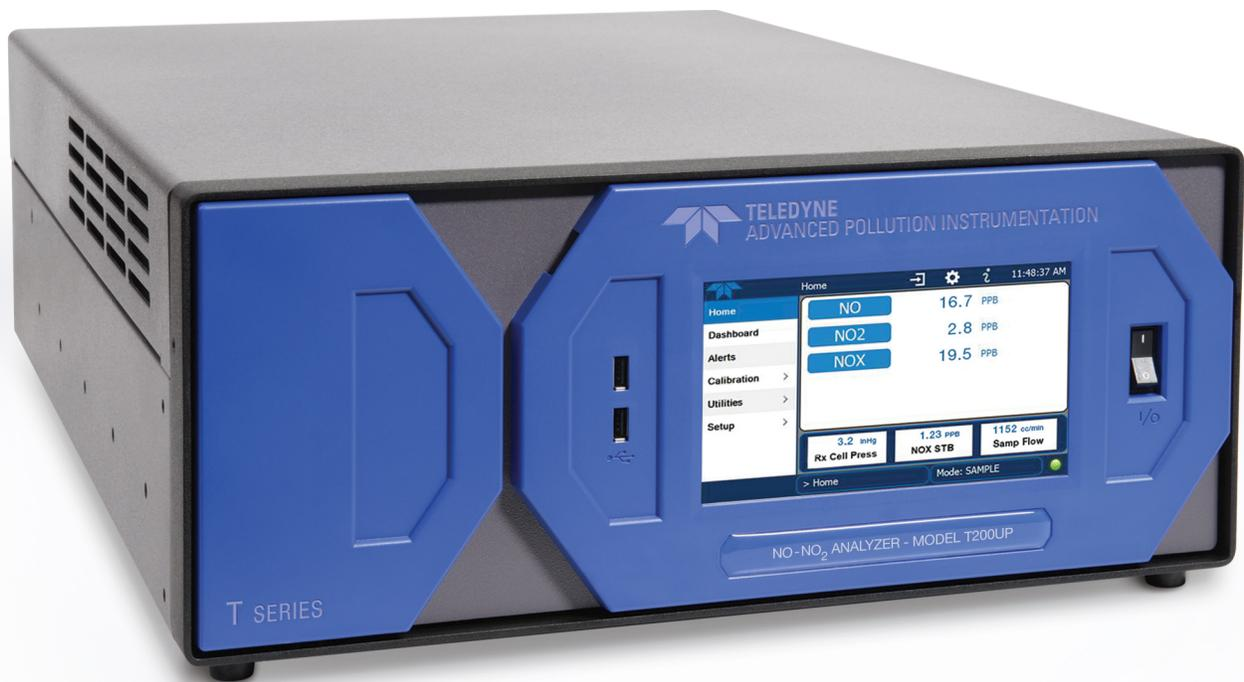
The Model T200UP provides Trace-Level measurements of NO, NO<sub>x</sub> and NO<sub>2</sub> using our Model T200U NO<sub>x</sub> analyzer combined with a patented high efficiency Blue Light Converter (BLC). The BLC, also known as photolytic converter, provides a very specific conversion of NO<sub>2</sub> with conversion efficiency similar to molybdenum.\*
