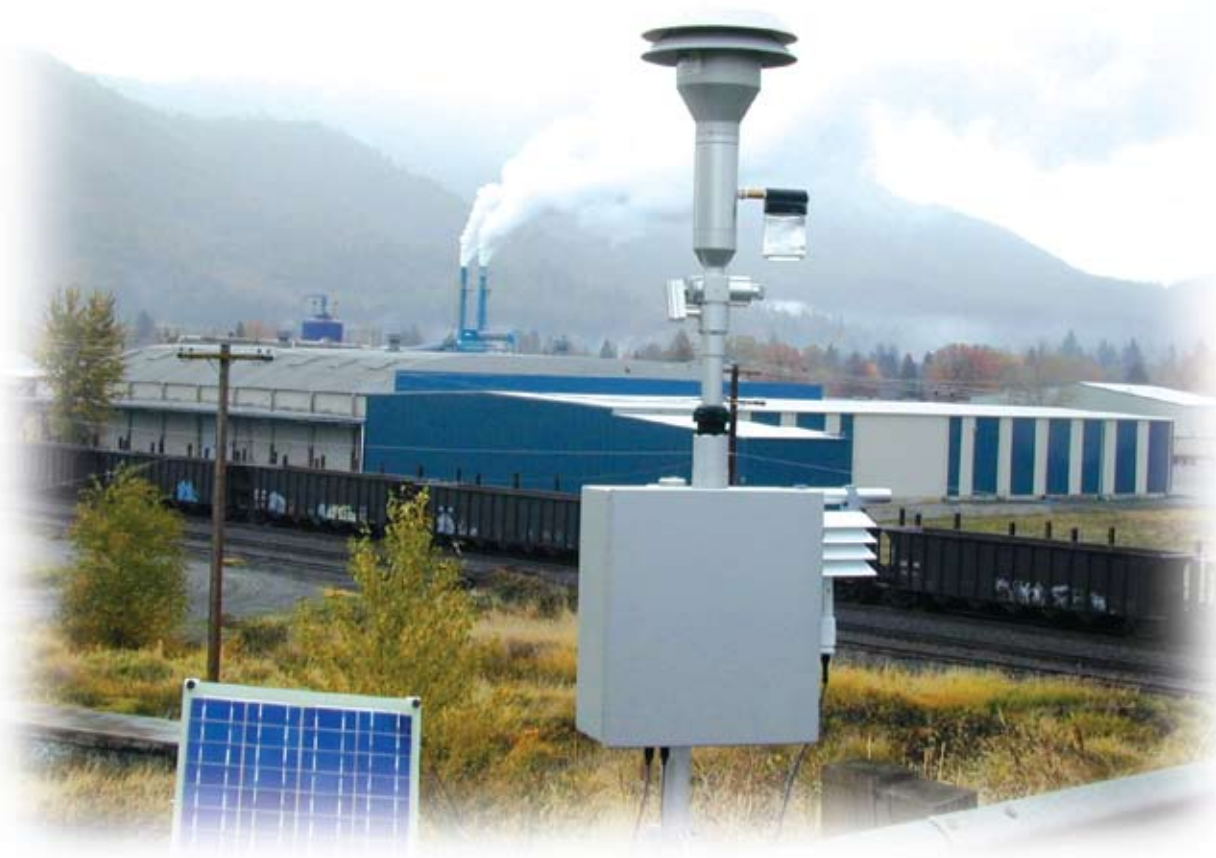
The Met One E-BAM is a portable, real-time beta gauge which is comparable to U.S. EPA methods for PM 2.5 and PM 10 particulate measurements.
