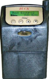
Flow Range 3 to 12 LPM Low Flows 50-800 cc/min with Low Flow Holder
