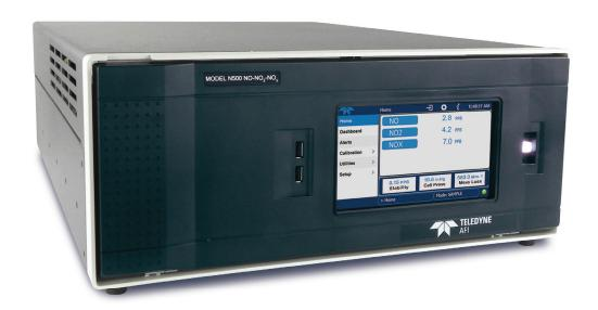
The Model N500 CAPS  $NO_x$  analyzer uses superior Cavity Attenuated Phase Shift (CAPS) Spectroscopy to measure True  $NO_{2'}$   $NO_{x'}$  and NO gases. The instrument combines direct  $NO_2$  measurements with highly efficient gas phase titration (GPT) to convert and measure the NO gas component. An automatic baseline reference cycle accounts and compensates for any potential baseline drift due to varying environmental conditions.
